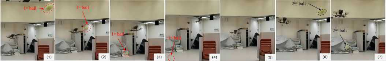
Fig. 9: Screenshots of the UAV dodging two balls thrown continuously while navigating the unknown environment. No mocap is used. The 2nd ball was thrown out in sequence (5) and the UAV successfully avoided it in sequence (6) and (7).
