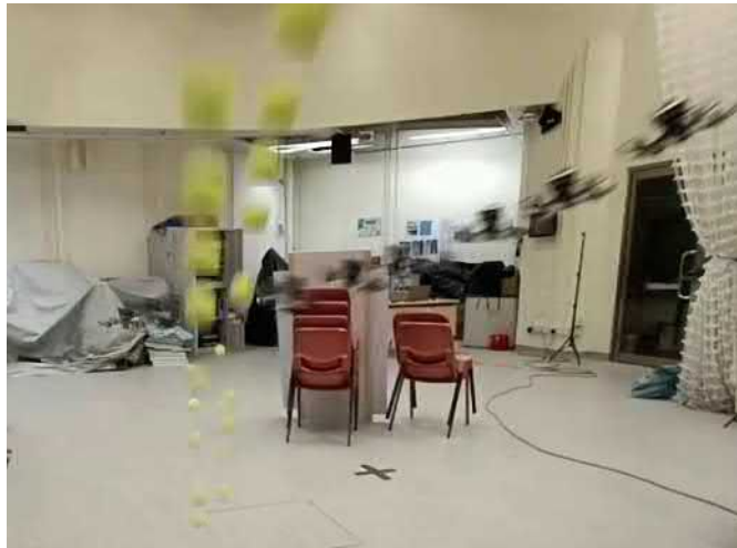
Fig. 1: Sequence of our UAV dodging the multi-balls attack. The two tennis balls are thrown out simultaneously. No motion capture is used.
